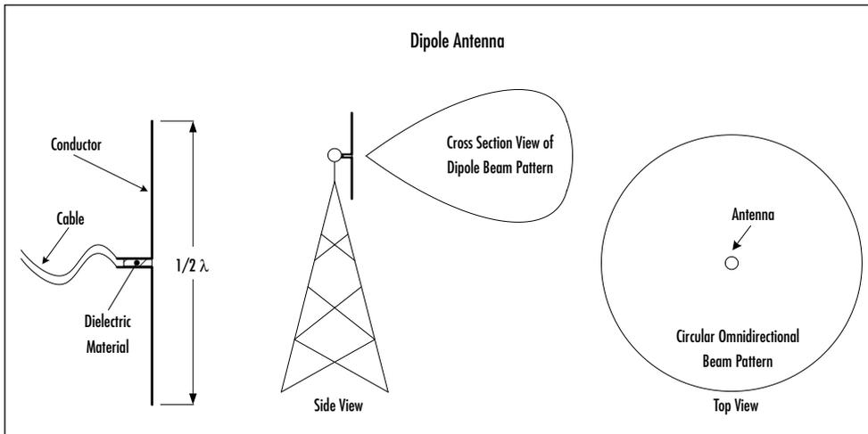
When the antenna is not near half the wavelength, the performance of the antenna is drastically affected due to a mismatch in characteristic impedances and standing wave ratios.
