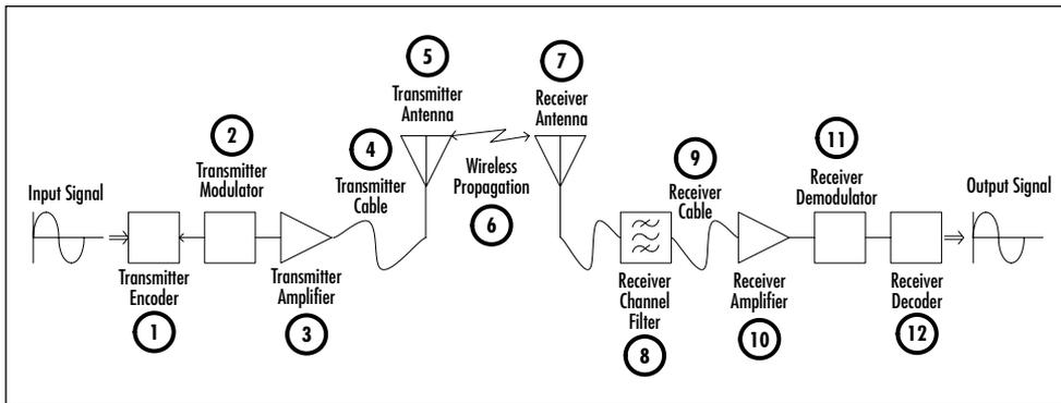
Each of the boxes in this picture represent entire subsystems of the radio; each is very complex, but simplified here as a box representing their function. The function of each of these boxes, following the system from the origin of the signal to the output of the receiver, can be described briefly as follows (refer back to Figure 2.13):
