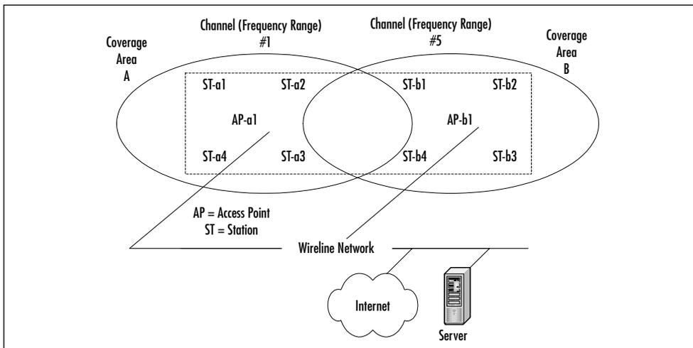
Since multiple Access Points exist in this model, the wireless devices no longer communicate in a peer-to-peer fashion. Instead, all traffic from one device destined for another device is relayed through the AP. Even though it would look like this would double the amount of traffic on the WLAN, this also provides for traffic buffering on the AP when a device is operating in a low-power mode.
