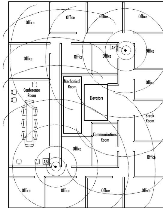
The access point wireless bridges will be placed on shelves near the antennas. The Ethernet ports of the access point bridges will be connected to the LAN switches that serve the floor. The LAN switch must be configured to permit multiple media access control (MAC) addresses on the data port.
