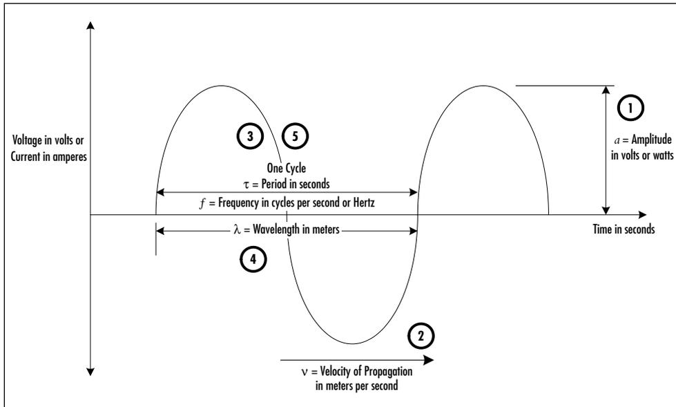
A *cycle* is the smallest portion of a waveform that, if repeated, would represent the entire waveform. Waveforms can be described as having the following properties (refer back to Figure 2.1):
