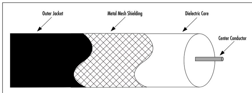
As mentioned earlier, the outer metal mesh of coaxial cable acts as a shield that shunts unwanted interference to ground. Since the shielding is tied to ground, it acts as a baseline reference. The center conductor carries the signal in reference to the outer, grounded shield. The spacing between the center conductor and the outer shield is very important and must remain constant; the dielectric material between the
