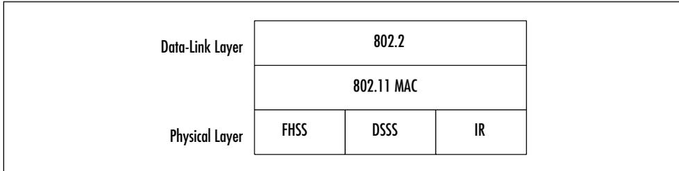
The three physical layer options for 802.11 are infrared (IR) base-band PHY and two radio frequency (RF) PHYs. Due to line-of-sight limitations, very little development has occurred with the Infrared PHY. The RF physical layer is composed of Frequency Hopping Spread Spectrum (FHSS) and Direct Sequence Spread Spectrum (DSSS) in the 2.4 GHz band. All three physical layers operate at either 1 or 2 Mbps. The majority of 802.11 implementations utilize the DSSS method.
