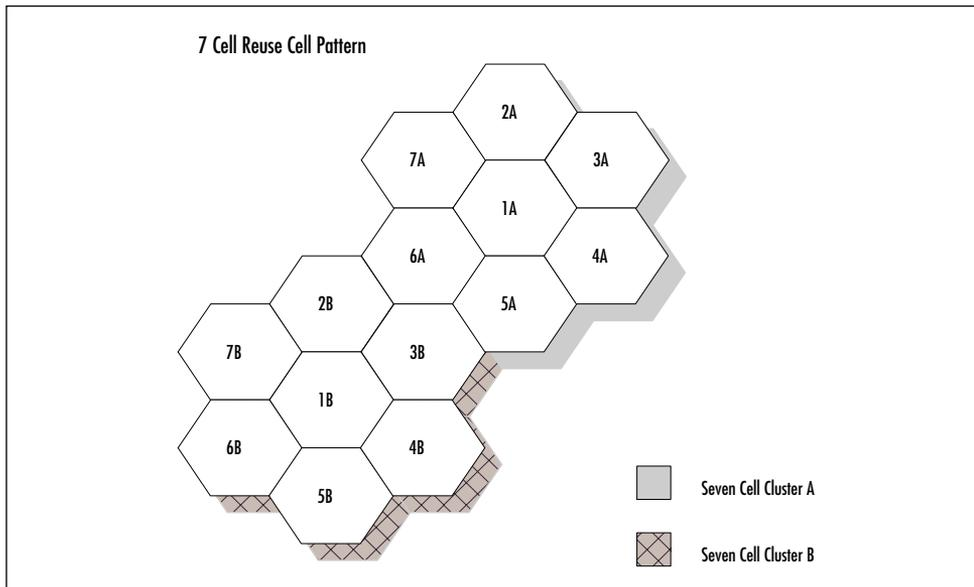
Each tower is made the center of its small coverage area, called a *cell*. Every cell is surrounded by six other cells, to form a honeycomb pattern. To prevent channel interference, the same channel cannot be used in adjacent cells. Once the signal has traveled the distance of 1.5 cells, it has been sufficiently attenuated so as not to cause interference to the main signals of that cell. Therefore, in every seventh cell, a channel could be reused.
