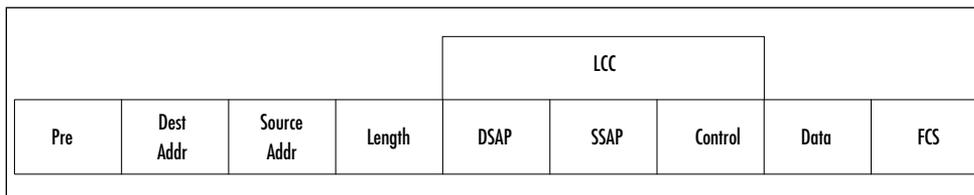
The frame format of the Ethernet packet includes the following fields:
