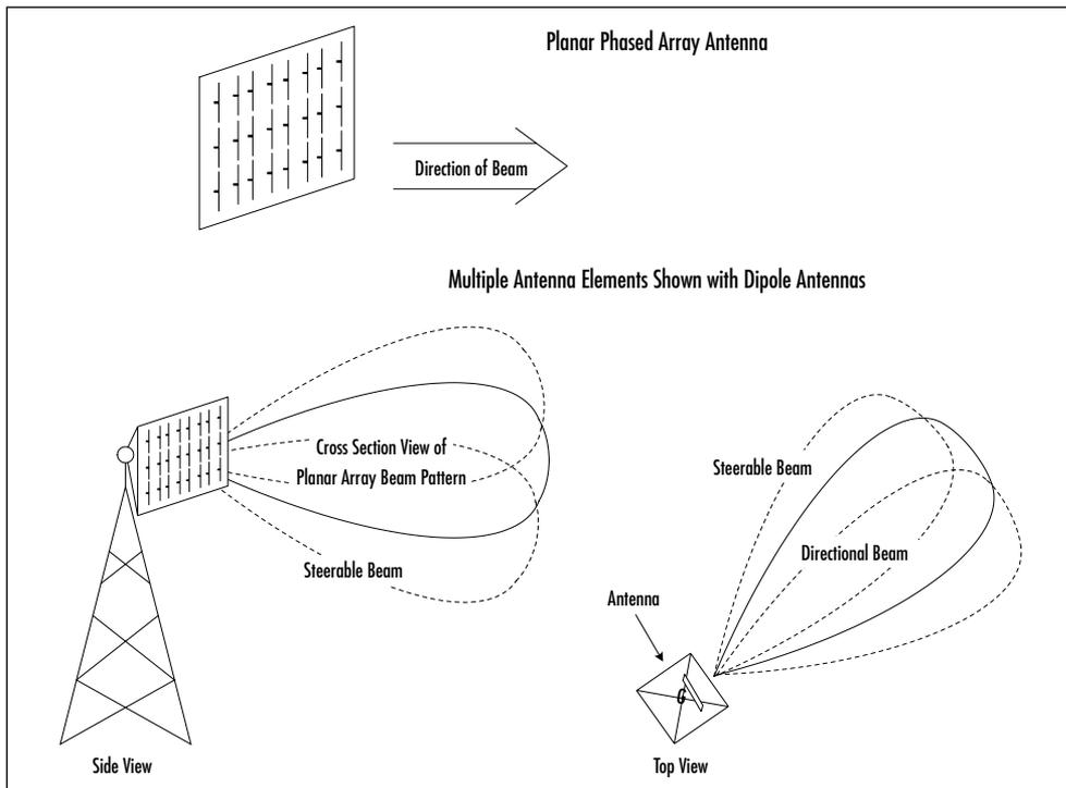
Planar arrays can have more than one active element. By changing the phase and power of the signal to hit specific active elements, the beam can be steered without the antenna physically moving. A useful application of this is on military tracking radars. A computer can adjust the input signals to the various elements of a planar array and steer the beam faster than the whole array could be moved physically, thus allowing for tracking of multiple fast-moving targets.
