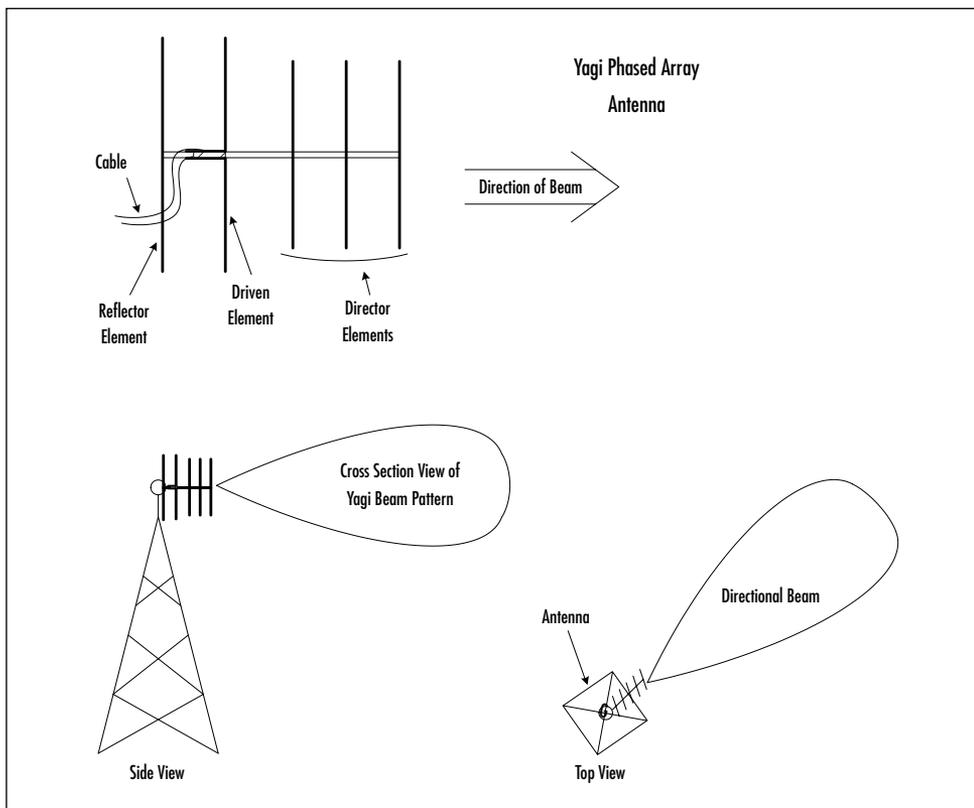
The elements are longest at the rear and gradually get shorter towards the front. The rear element is called the *reflector*. Immediately in front of the reflector is the *driven element*. In front of the driven element are one or more *director* elements.
