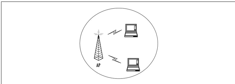
single radio cell. If there are no connections back to a wired network, this is called an *independent basic service set*.
